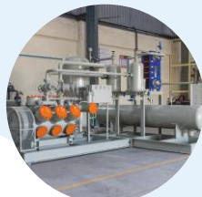
Skid mounted refrigeration units
