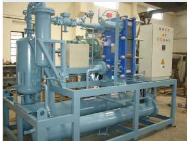
Screw Compressor Condensing Unit
